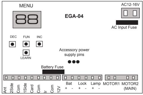
**Tip**: Green connector blocks on the main control board can be removed to help with wiring in cables
