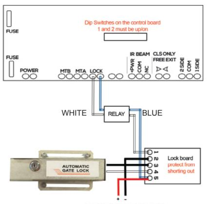
PICK UP POWER FROM SOURCES AVAILABLE (BATTERY, CONTROL BOARD, REGULATOR IF SOLAR, ETC)
