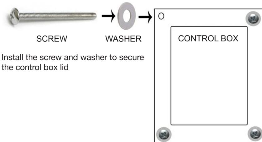
Install the screw and washer to secure the control box lid
