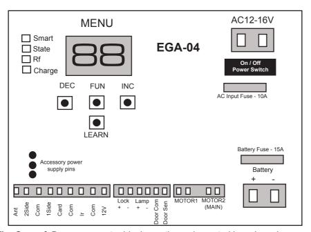
**Tip**: Green & Brown connector blocks on the main control board can be removed to help with wiring in cables
