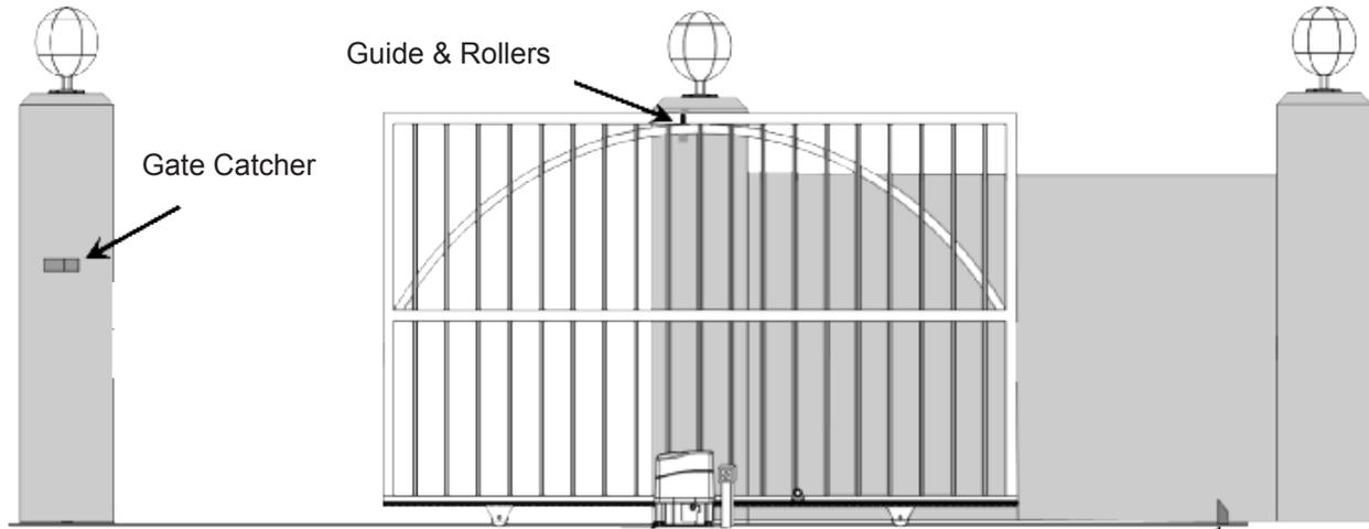
Important - the gate MUST have permanent end stops in both the closed and open positions to prevent the gate running off the track in the even of a failure
