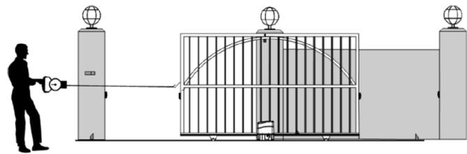
**Pull Force:** place the gate in the fully open/closed position and pull on the scale until the gate starts moving. The value showing on the scale at the point that the gate starts moving is the Start up Force kgf.
