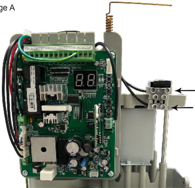
Bring low voltage cable up through the hole in the baseplate. Push the wire through one of the 2 inlets (see image B). Put wire through cable locking tab. Now screw the wires into the connector as show in image A
