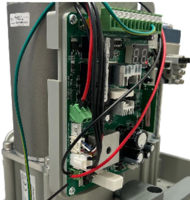
Black negative wire and red positive wire connected to battery terminal on main board
