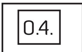
The LED display shows the current consumption of the motor. "0.4" During the system learning procedure, the control panel will automatically detect the current consumption from the motor and indicate the resistance level of the gate while the motor is in operation. If this reading increases instantly or stays in the high readings, please check the running of your gate such as wheels, track, rack etc.
