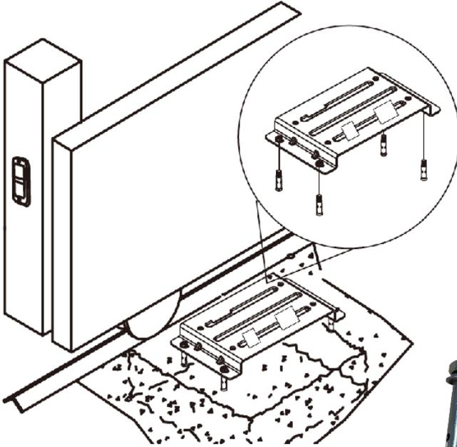
1. Lay a concrete slab 400mm x 400mm x 200mm
